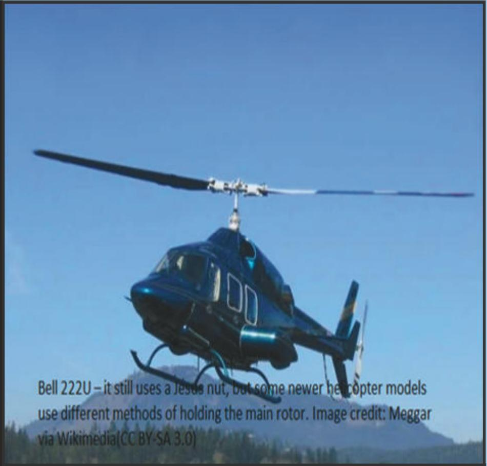
Bell 222U – it still uses a Jesus nut, but some newer helicopter models use different methods of holding the main rotor. Image credit: Meggar via Wikimedia(CC BY-SA 3.0)
